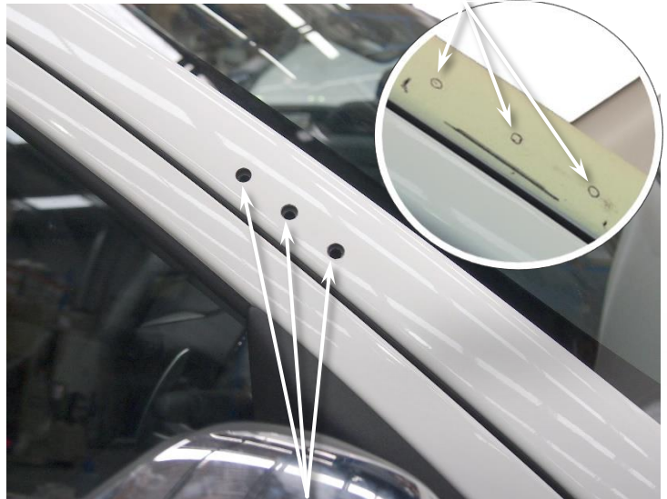
Drill A-pillar Panel 8mm, Inner Panel 6mm
